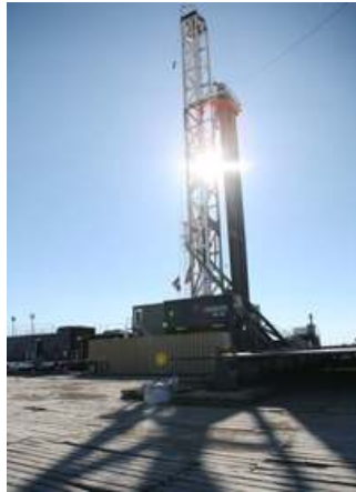
The raised platform used by Encana at some of its drill sites helps to protect the underlying landscape. (Credit: Abrahm Lustgarten/ProPublica)
